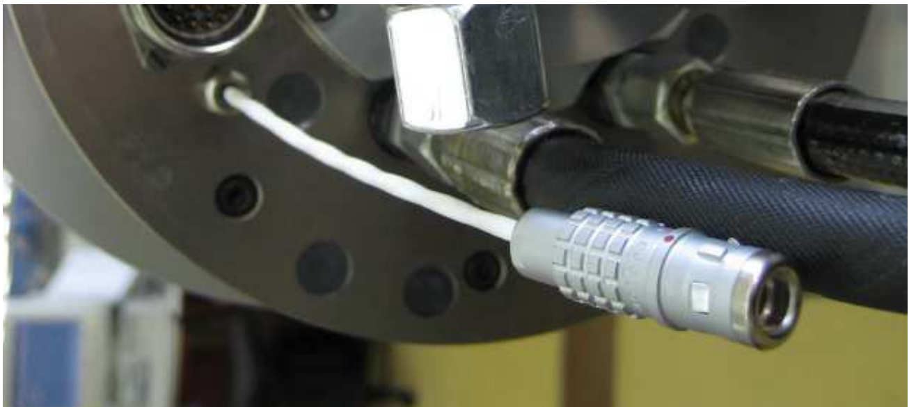
Sensor connector with section of cable on the end of the spindle
