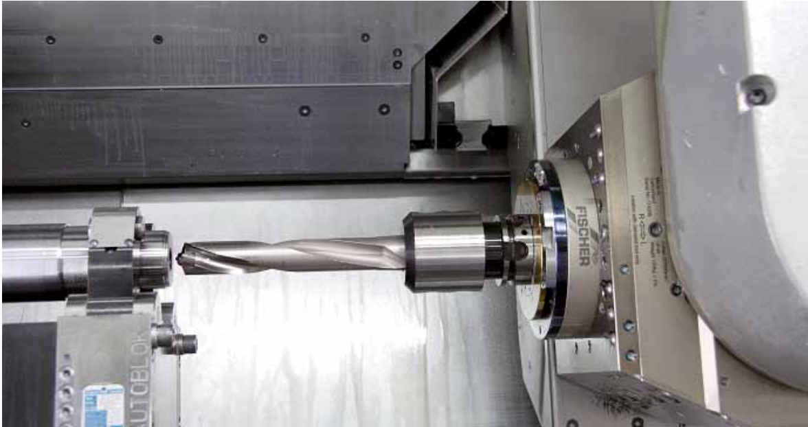
Image 6: Use of the spindle MFW-2104/24 of the CSC series in a DMG GMX 400 LINEAR turning/milling centre
